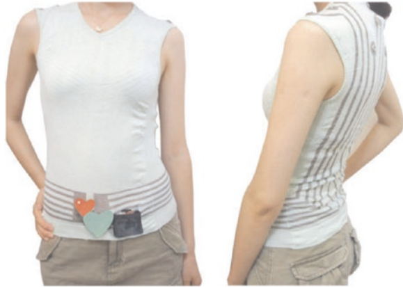
Fig. 7.10 Prototype garment having TENS function
