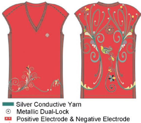
Fig. 7.11 Innovative design pattern of intarsia for routing hiding based on garment prototype [12]
