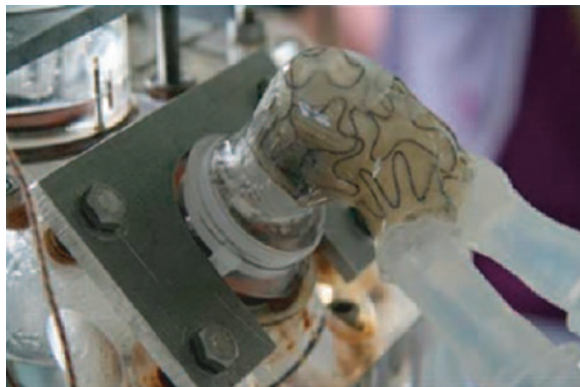
Fig. 20.4 Prosthesis in the circulatory simulator [18]
